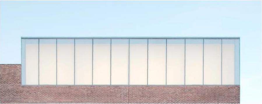
In contrast to the brick below, second floor of the CSB will be visually lighter with extensive glazing, translucent and opaque panels
