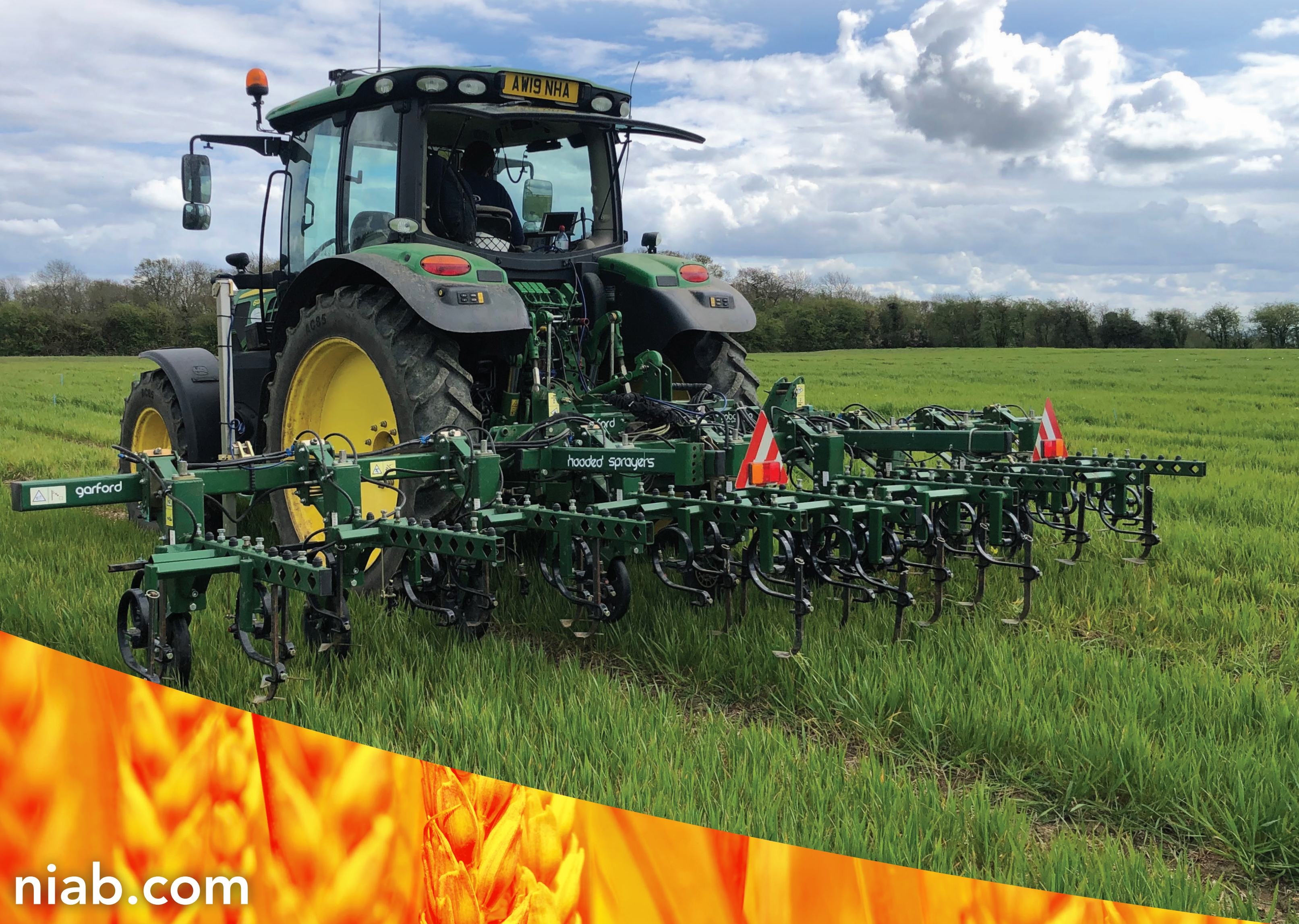
Figure 1. Cultivate inter-row spaces before crop stem extension; careful machine set-up minimises undercutting crop
