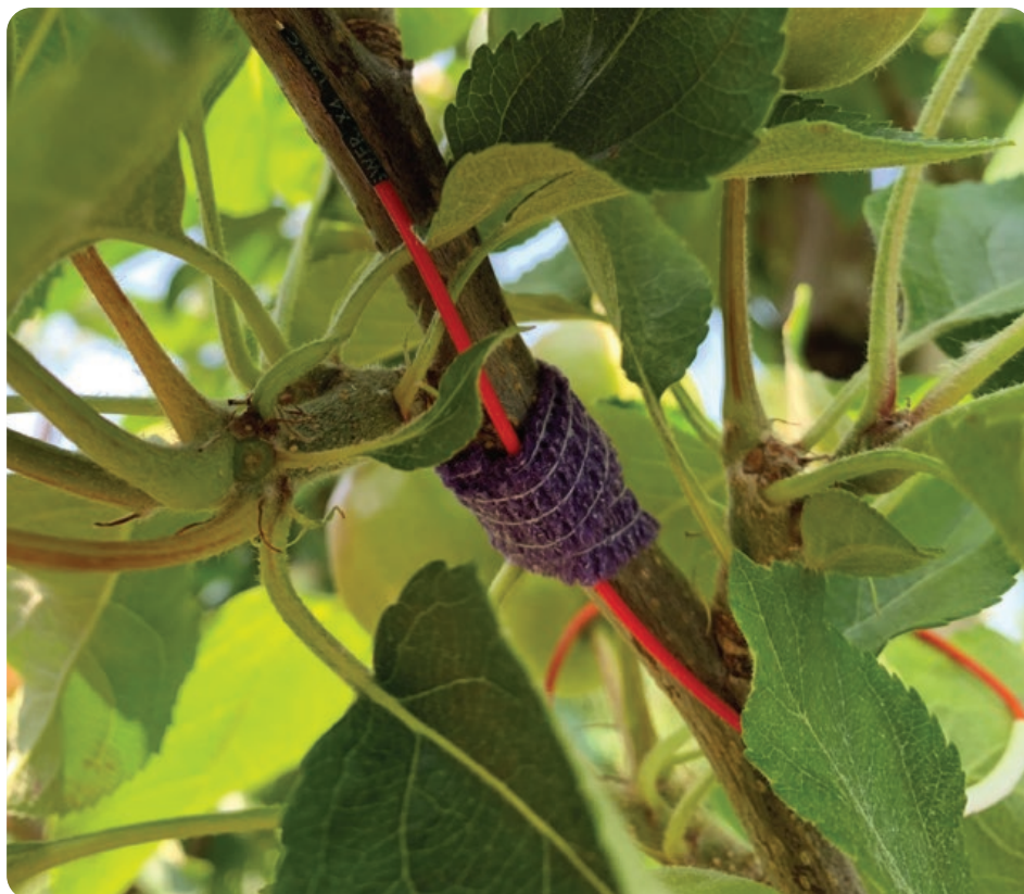
Figure 3. Sensors are inserted in the branch vascular system
