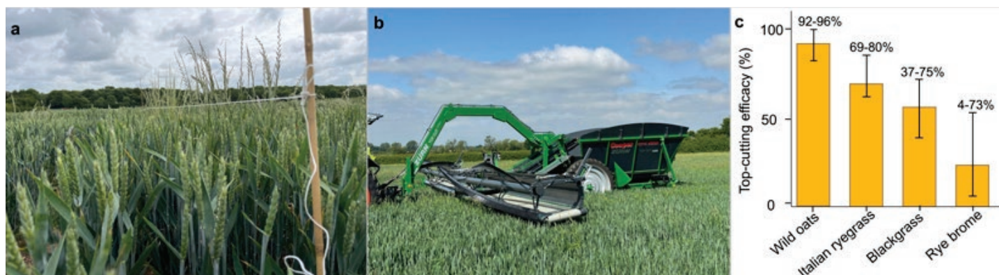
Figure 3. (a) Experimental simulation of a top-cutting machine showing cutting height threshold indicated by a string set above wheat canopy, (b) Zürn's commercial Top-Cut Collect machine, and (c) top-cutting efficacies by species, averaged across wheat variety, cutting treatments, and seasons
