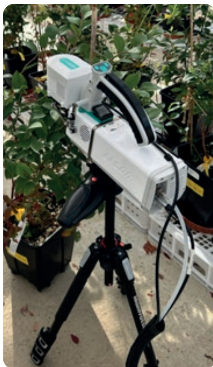
Figure 2. Licor device measuring chlorophyll fluorescence
