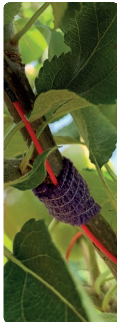
Figure 3. Sensors are inserted in the branch vascular system
