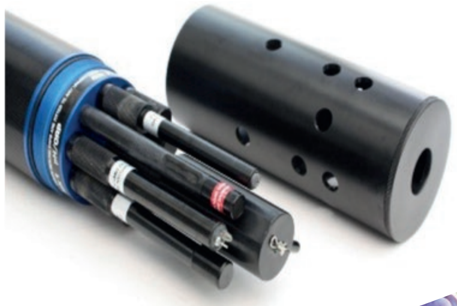
Figure 3. Sonde technology to measure NPK leaching
