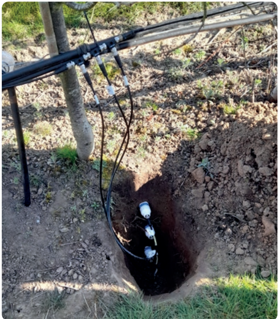
Figure 1. Measuring N, P and K at different rooting depths
