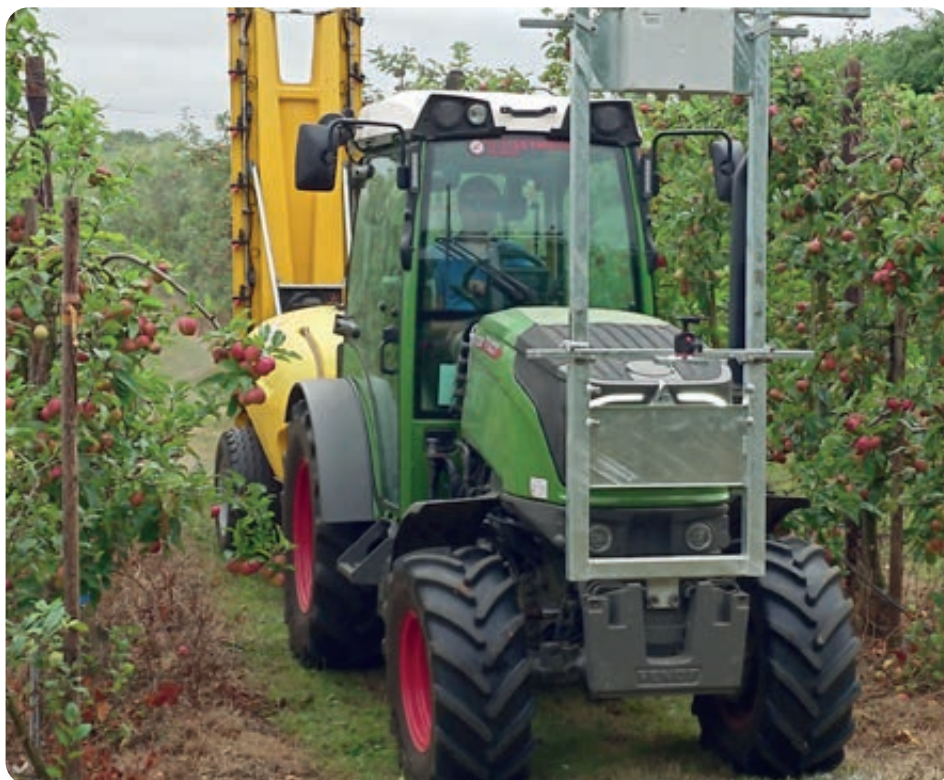
Figure 2. The sprayer applies adjusted doses to individual trees
