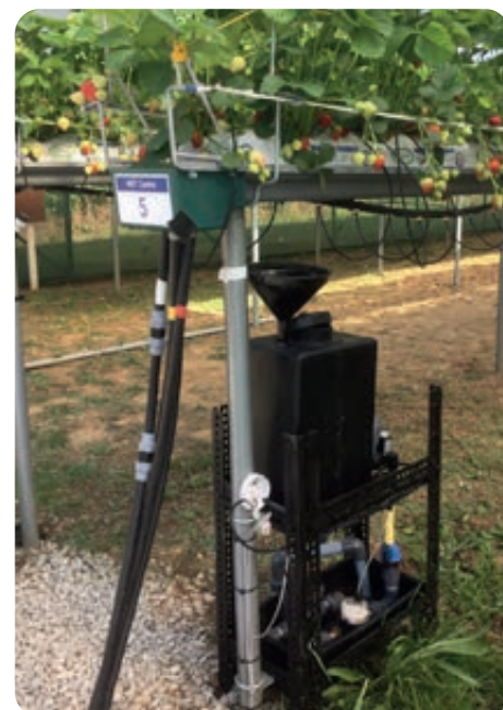
Figure 2. Measuring run-off from bags at the WET Centre
