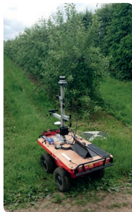
Figure 3. Antobot 'scout' robot collecting data to develop systems for autonomous navigation
