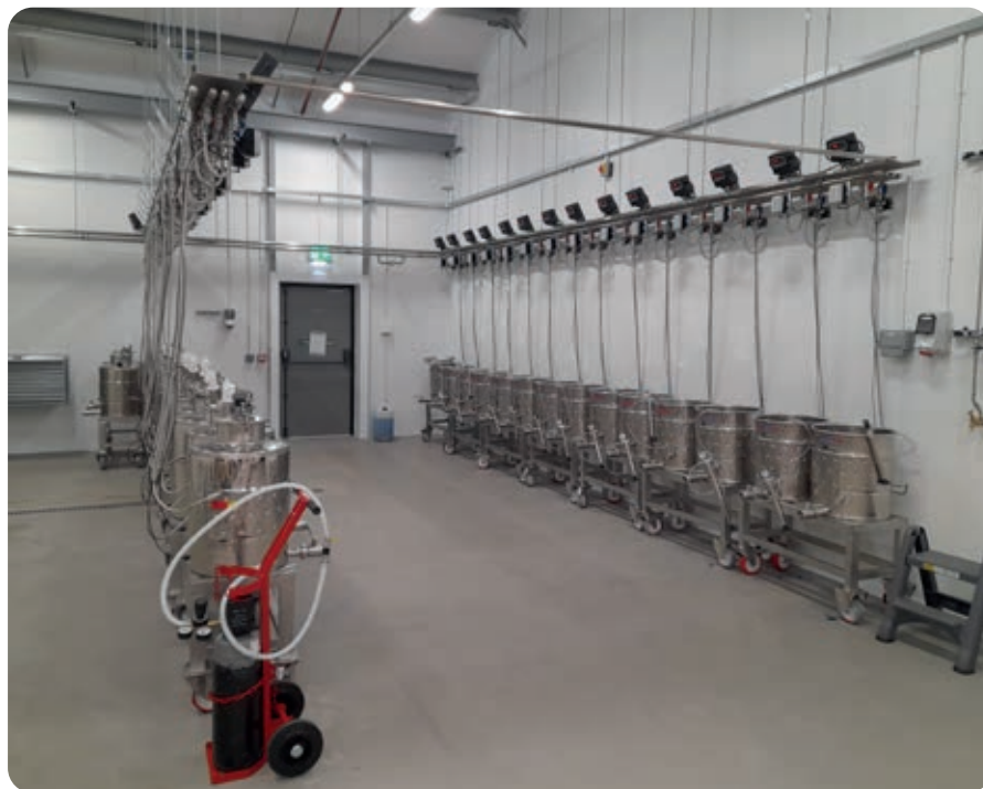
Figure 2. The fermentation tanks have automatic temperature control
